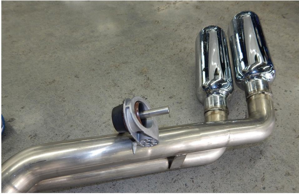
**Step 4:** Slide (2) 2.25" clamps over the expanded tailpipe inlets then slide both expanded inlets over the muffler outlet pipes. Snug the clamps do not tighten!
