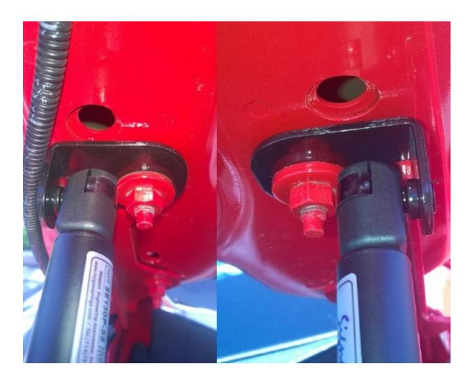
Step 3. Tighten the nuts to secure the bracket and hood hinge.
