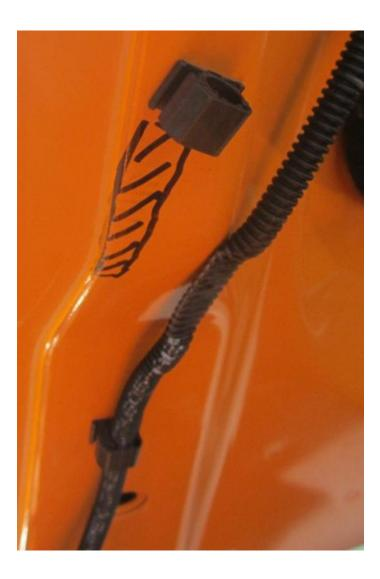
Step 10. Release both clips. Remove hose from both clips. Move hose downward about ½" & re-fasten lower clip. Interference area as marked.
