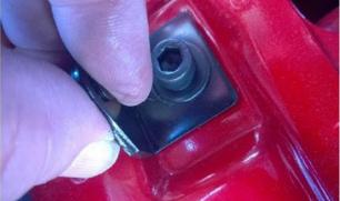
Postion the brackets by putting the serrated washer inside oval fender hole.
