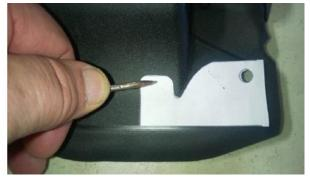
Step 5. Cut 1" hole with center in the marked location. CAUTION DO NOT USE a spiral drill bit
