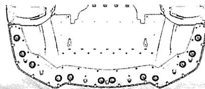
8. Install (21) plastic rivets (W704342-S300) to attach the Performance Plus Splitter (JR3B-17D997-A\*) to the Lower Valance and Belly Pan, using a POM rivet tool.
