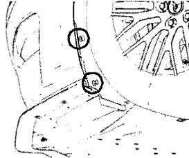
*\*Note: Push-pins should be set aside as spares. Replacement push-pins included in kit.*
