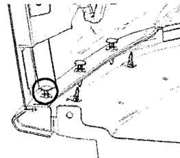
*\*Note: Push-pins should be set aside as spares. Replacement push-pins included in kit.*
