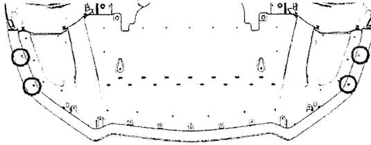
2. Remove (4) screws (W715060-450B) on outboard edges of Belly Pan.
