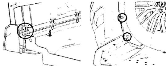
7. Install (12) screws (W715060-S450B) to attach the Performance Package Level 2 Splitter (JR3B-17D997-A\*) to the Lower Valance and Belly Pan. Tighten screws securely (reference torque 1.9Nm).
