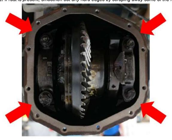
7. Install differential housing cover and gasket using bolts supplied in the differential housing cover kit (10) and the two (2) brake cable retainer studs.
