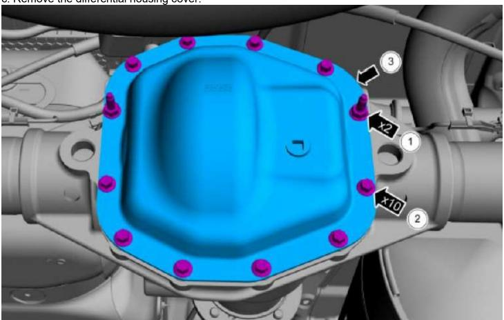
4. Remove differential cover gasket, discard after removal.
