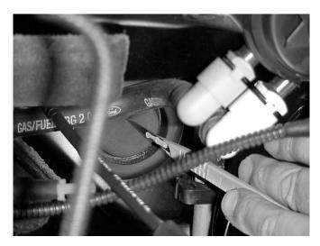
STEP 2: Snake the 1/8th inch hose from your kit through the grommet and into the passenger compartment. Run the hose along the steering column and under the rubber flap.
