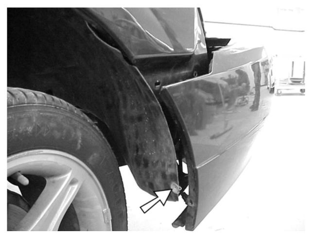
Note: Turning the wheels to the right to remove the left side screws and to the left to remove the right side screws will make the removal easier.
