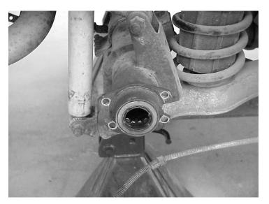
**STEP 13:** Reusing the backing plate bolts, install the caliper to axle adapters (item 38 and 39). Torque bolts to 45-50 ft./lbs. Axle adapters are marked LH and RH. The RH is shown below.
