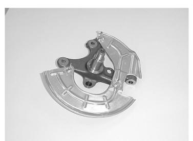
**STEP 20:** Install new spindle (Item 1 RF and Item 2 LF) over ball joint stud and place ball joint spacer (Item 23) on ball joint shaft.
