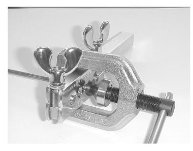
**STEP 12:** Back off the flaring cone slightly, remove the adapter, and then screw cone down again tightly, this time directly into the tubing. This folds the tubing back on itself forming an accurate 45° double-flare.
