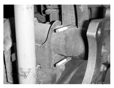
**STEP 27:** Slide the caliper brace into place over the U-bolt as shown and loosely install the nuts.
