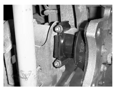
**STEP 28:** Install new rear rotors (Item 45) on the axle using a lug nut to temporarily hold the rotor in place.
