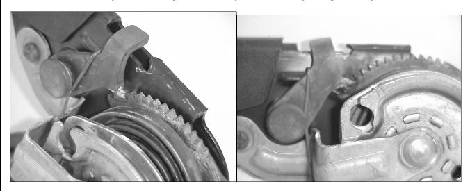
**STEP 8:** Drill out the center hole in the rear cable equalizer to 11/32" diameter.
