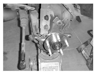
**STEP 27:** Reconnect the tie rod ends and install the nut. Torque to 35-47 ft./lbs.
