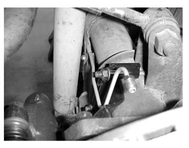
**STEP 34:** Unbolt the lower shock mounting hardware and wire the shocks out of the way toward the center of the car. Using the hose bracket (Item 27 RR and Item 28 LR) as a guide, mark and drill a 9/64" hole (position 1 shown below) for the bolt and a 11/32" hole (position 2) for the bracket guide tab. The installed bracket position should as shown.
