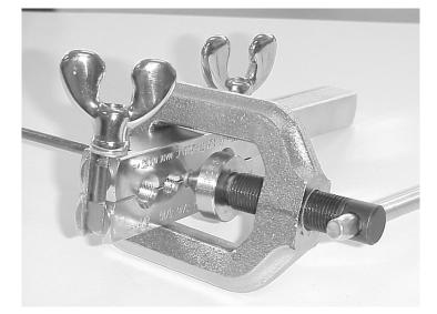
**STEP 9:** In step 1, the 7/16" tube nut is slid on the line and the line is placed in the proper hole in the flaring bar and the wing nuts tightened. The end of the tube should protrude above the top of the flaring bar by a distance equal to the thickness of the shoulder on the 7/16" adapter.
