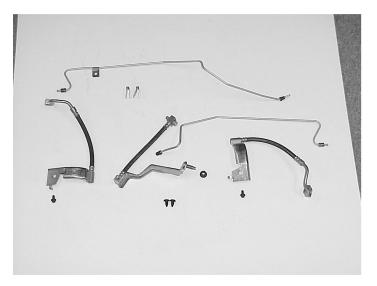
**STEP 32:** Install the new body to axle hose bracket (Item 34) on the rear axle housing in the position shown. **Note: Do not install the nut until after the wheel lines are connected.** Connect the banjo fitting to the main brake line. Torque to 30-40 ft./lbs.
