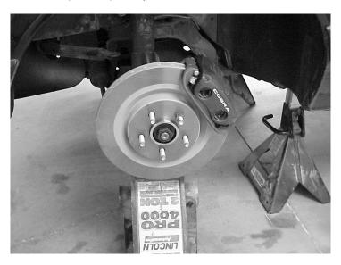
**STEP 29:** You will also have to move the right front brake tube approximately 1" forward. Re-drill the holes for the clip alignment tab (1/4"diameter) and screw (3/16" diameter) using the clip as a template for hole location. Install the mounting clip using the original self-tapping screw. Install front brake hose in the mounting clip.
