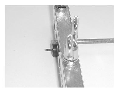
**STEP 10:** Insert the 7/16" adapter in the brake tube.
