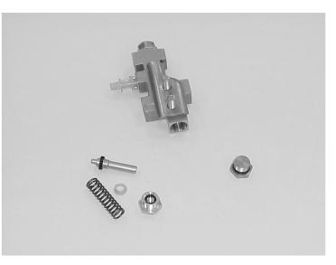
**STEP 3:** Remove O-ring from old valve plug and install the O-ring on the new valve plug (without hole--Item 26). Install the new plug (Item 26) in the new proportioning valve.
