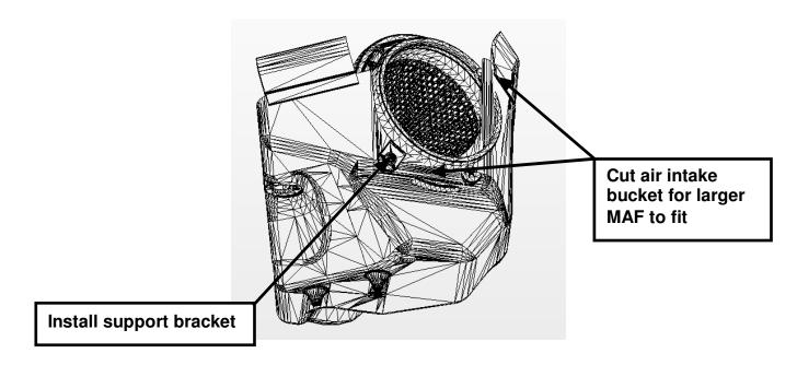
STEP 4: Lower the complete air intake bucket assembly into the vehicle using the two pegs as guides into the rubber grommets. Use the new air intake bucket bolt and newly supplied J-clips to secure the air intake bucket in the vehicle. Torque the M6 bolt to 8 Nm (70 lb in).
