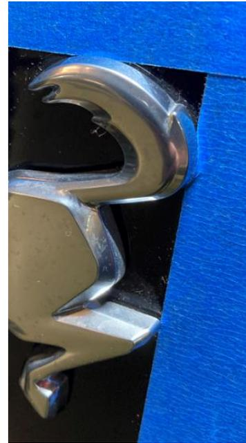
2. Use a heat gun or hair dryer to loosen the adhesive on the back side of the emblem.
