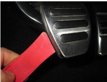
**STEP 7:** Repeat the process outlined in STEP 6 to install the clutch pedal cover.
