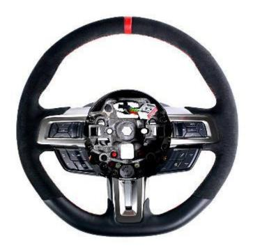
NOTICE: If vehicle is equipped with a heated steering wheel option, you will lose functionality of this feature after installing the M-3600-M350RA Mustang GT350R Steering Wheel
