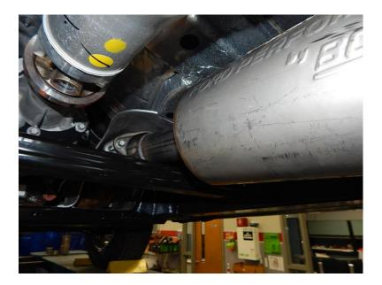
STEP 2: Install the proper "Mid Pipe" for your wheel base. Be sure to slip a clamp onto the pipe, clamp to be tighten later.
