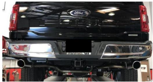
Step 12: Once you are satisfied with your fitment, check for clearance to all body and vehicle components, especially the spare tire heat shield and wiring around the rear axle. Torque all clamps to 48 N-m. (35 lb-ft)
