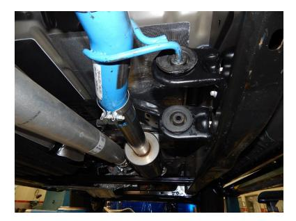
Step 4: Place clamp over mid-muffler inlet and install. First place tailpipes over rear axle, then slide expanded inlet over the s-pipe and the hanger into the rubber isolator.
