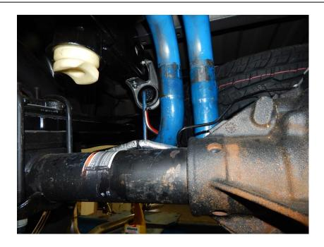
Step 7. Adjust tips to side of truck, with minimum  $\frac{1}{2}$  gap on top of the tips.
