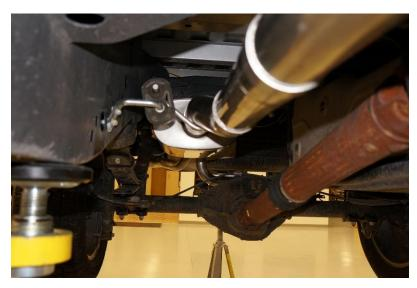
Step 6: Heat Shield installation. Drop the spare tire per the vehicle owner's manual instructions. Place the (2) J-nuts into the square holes on top of the cross-frame rail. Work the lip of the heat shield over the frame rail. Attach with (2) bolts provided. Using a 13mm socket torque to 20 N.m (15 ft-lb).
