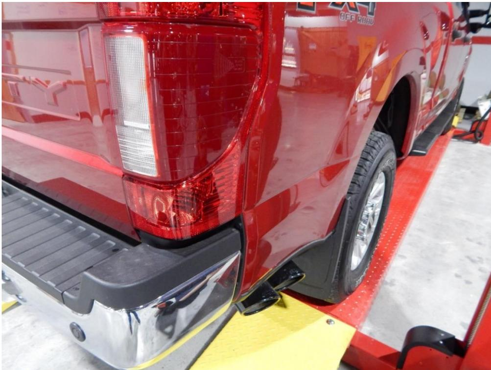
**Step 7:** Once you are satisfied with your fitment torque all clamps to 48 N.m. (35 lb-ft). Check clearances to wires, brake lines, and body parts.
