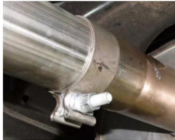
**Step 6:** Adjust tips to the side of the truck, with minimum ½' gap on top of the tips.
