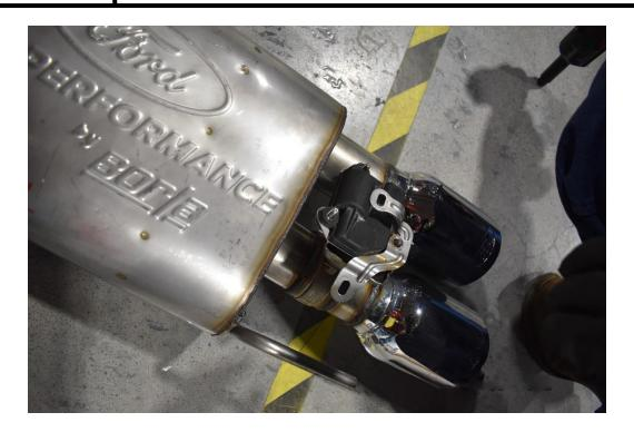
Step 5: Install supplied clamps onto the new muffler inlets and slide muffler hangers into factory exhaust hangers. Next slide the mufflers over the under axle pipes, centering tips in rear bumper opening. Attach the wiring harness to the valves if applicable.
