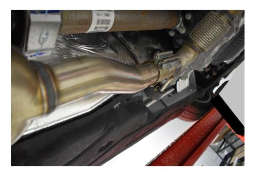
Step 2: Install factory hangers (previously removed) onto under axle pipes.
