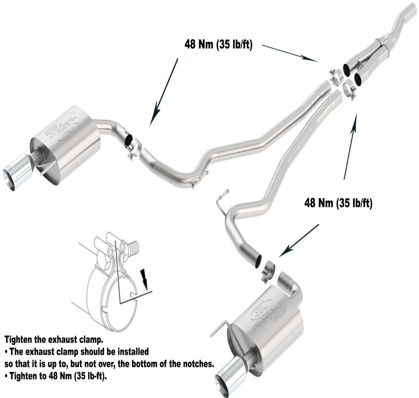
**Tighten the exhaust clamp.**
