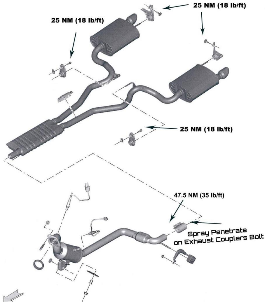
**STEP 3:** Using a 15mm socket loosen nuts on clamps (See Fig. 3).
