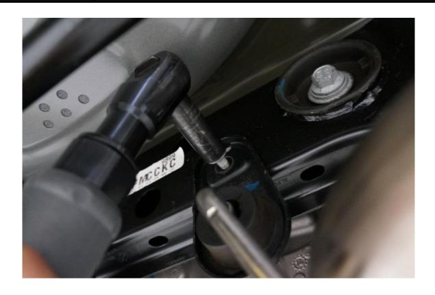
Step 5: Using a 13mm socket tighten bolts to 25 nm (18 lb-ft) in rear Sub frame exhaust hangers.
