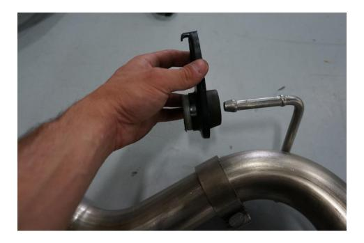
Step 4: Install supplied clamps onto front muffler side of under axle pipes, slide pipes/clamps onto front muffler. Using a 13mm socket install bolts in exhaust hangers in rear sub frame.
