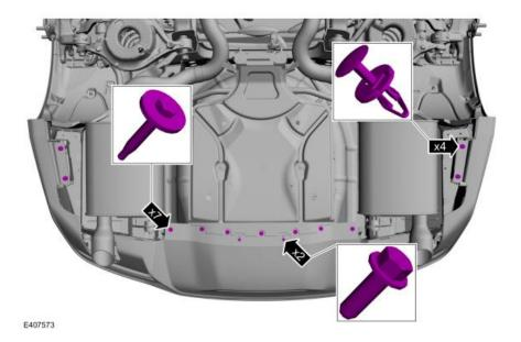
On both sides.Remove the screw, the push pins and position the wheel liner aside.
