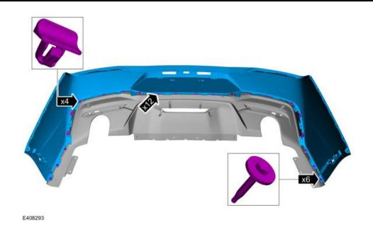
17. install the provided valence by snapping together clips and reinstalling bolts from step 151. Do not reinstall rear bumper until Exhaust modification is complete and installed.
