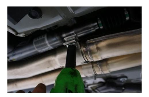
STEP 5: Using a 13mm socket to remove bolts from exhaust hangers in rear Sub frame near the rear axle, LH and RH sides.
