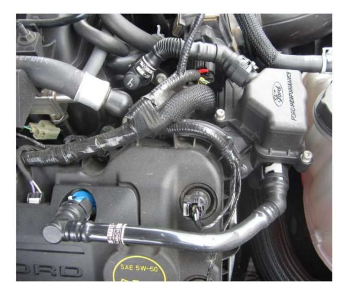
Maintenance is based on the type of driving the vehicle is subjected to. Track type driving will require more frequent checks for accumulation of oil in the separator. Remove separator and tilt so to empty oil out from the lower fitting. Do not empty from upper fitting! If removal of the top cover is required, when reinstalling, torque socket head screws to 4.5 to 5 Nm.
