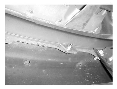
STEP 12: Attach fascia support to lower fascia with supplied fasteners as shown in the figure below.
