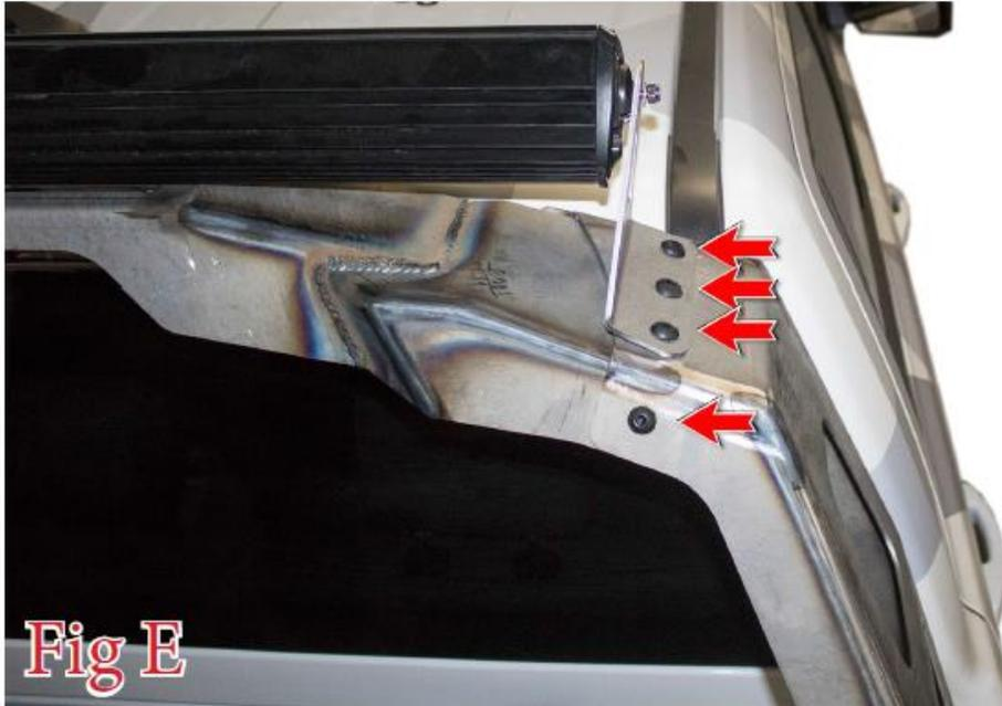
9. Hold the chase rack side pieces straight as you go back and tighten the mounting bolts. Tighten the 1/2" mounting bolts to 57 lb-ft. Then, tighten the M8 mounting bolts to 22 lb-ft. (Fig F)
