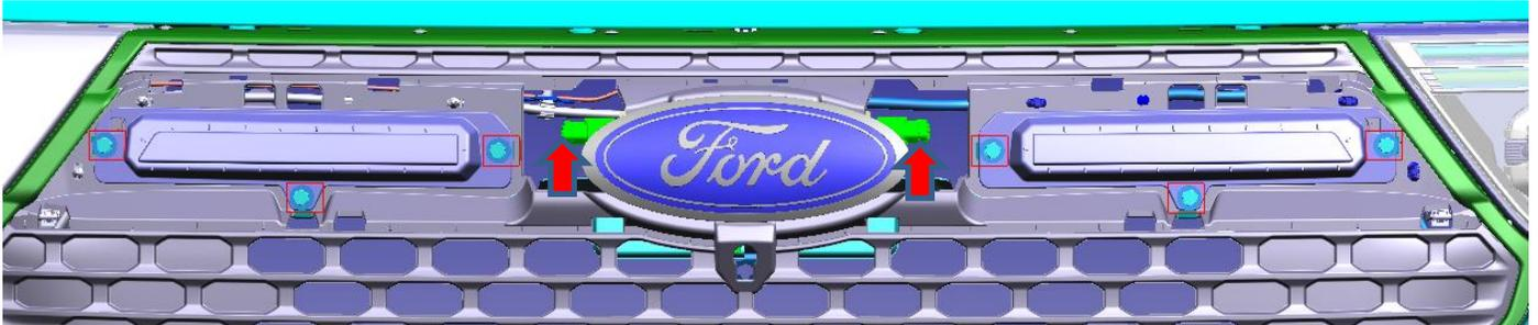
3. Plug light pigtail (not shown) into harnesses (x2). Hide the wirings behind light assemblies. Install aux lights into grille using the original fasteners.
