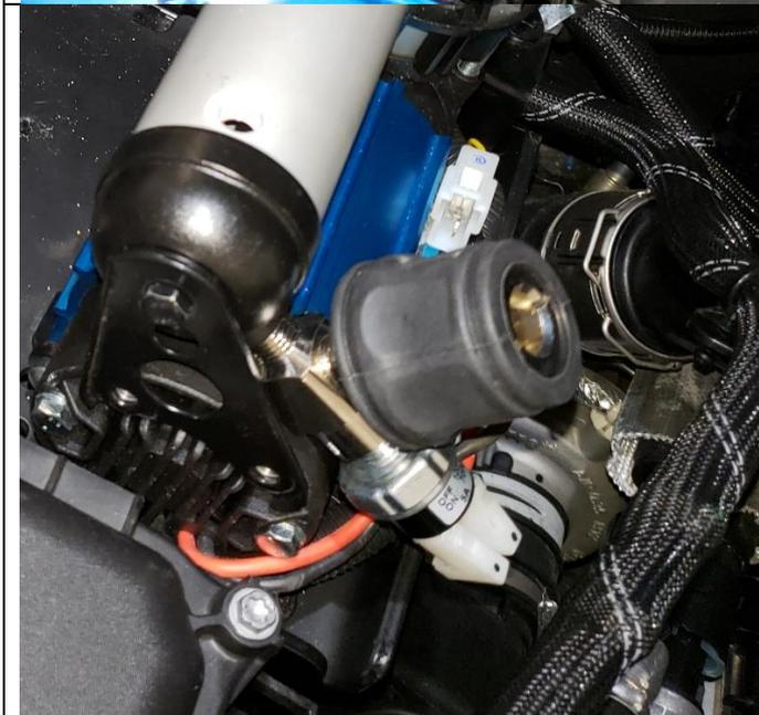
67. Install pressure switch and air chuck.
