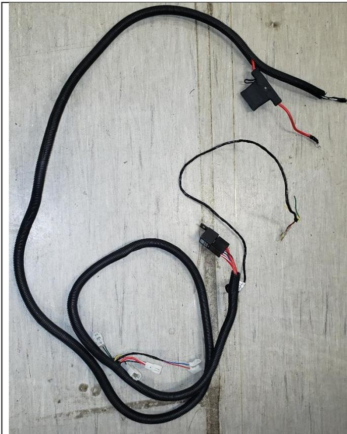
53. With the two cut sections of the wiring harness, reverse and reattach (the section with the fuse) by soldering the exposed ends to the ends of the other section that were cut in the previous step.
