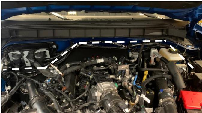
60. Pickup power from the stability bar module fuse (10A) located in the engine bay fuse box. Fuse reference #158 in owners manual.
