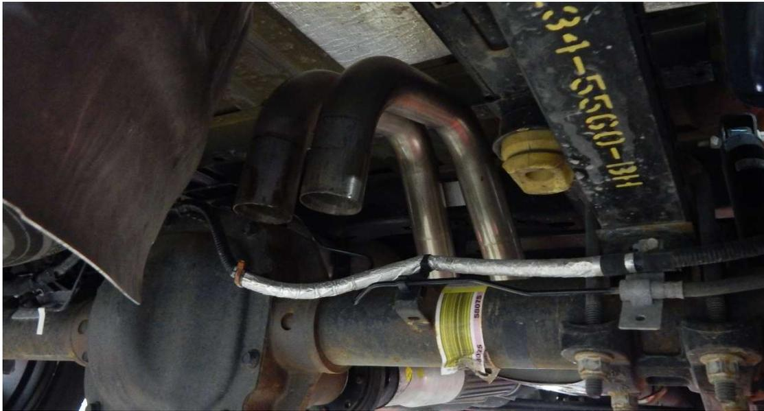
**Step 3: Remove the tailpipe isolator from the frame (2 bolts, use 10mm socket). Slide a 2.25" clamp over each inlet of the tailpipe assy, and slide the tailpipes over the muffler outlets. Reattach the isolator to the frame using the 2 factory bolts. Do not tighten the clamps.**
