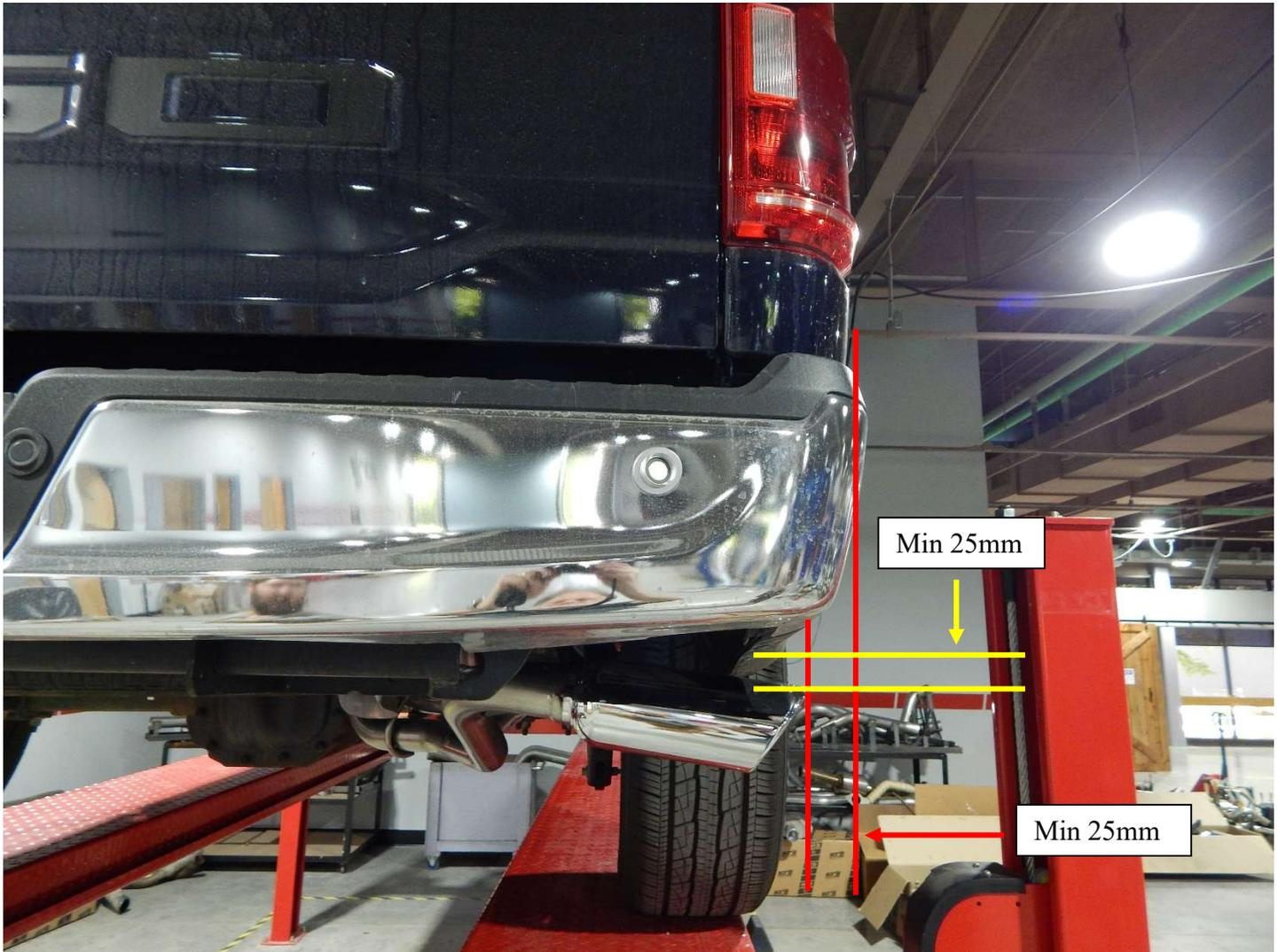
**STEP 5: Start vehicle and check for any leaks. If any leaks are found, determine cause (such as loose or incorrectly positioned clamp) and repair as necessary.**
