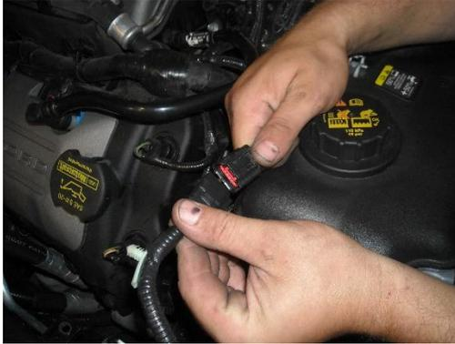
**STEP 43:** Clip the remaining (2) connectors on the jumper harness to the throttle body.
