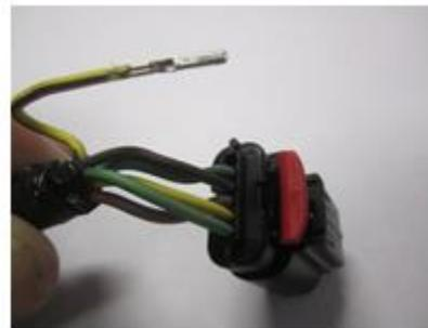
**STEP 41E:** Prepare the NEW replacement connector for terminal insertion by removing the red retaining lock from the connector. Like the previous connector, this lock can also be removed by gently prying out.
