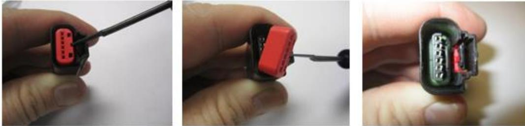
**STEP 41C:** Starting with Pin 1, carefully pry back the plastic retaining tab (which holds the female terminal into the connector housing) while gently pulling on the wire from behind until the terminal has been released.
