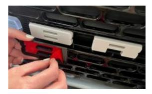
4. Position the overlays over the factory part starting from the top edge then downward, ensuring it is centered properly. Press lightly to adhere.
