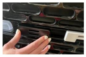
5. Using a lint-free scratch resistant cloth, press firmly on the overlays from the center working outwards to the edges to ensure maximum adhesion contact.
