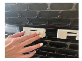
2. Before removing the adhesive, check fitment of the overlays on the factory parts.
