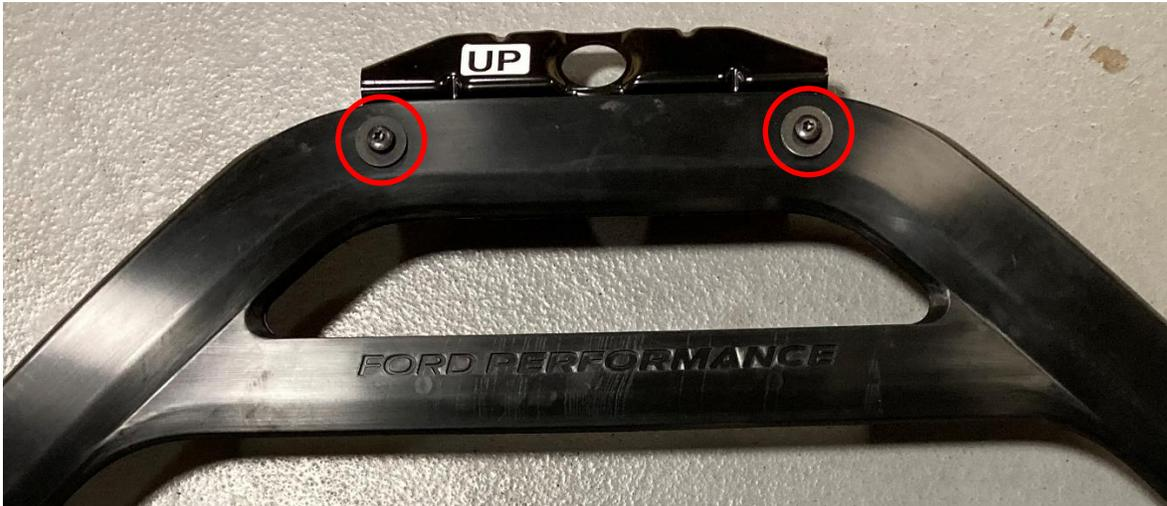
2. Install the J-clips (M8) on the rear header, as shown in the image.
