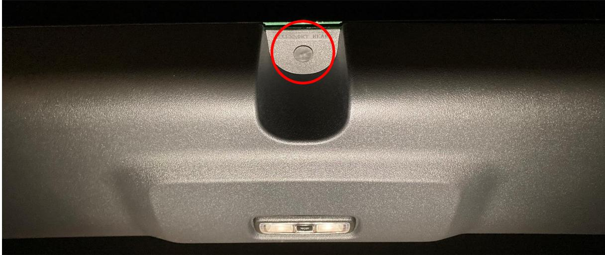
2. Disconnect the electrical connector for one side of the curtain airbag.
