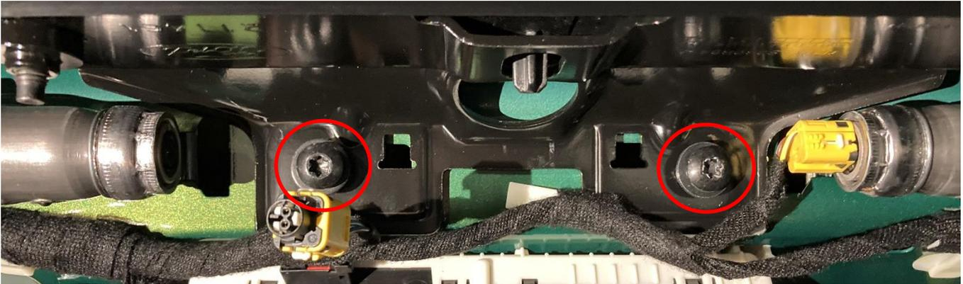
4. Install the C-bow brace to the side pillars using the bolts and washers (M8x30).
