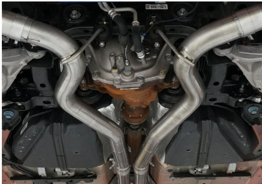
11. Place two (2) of the provided Exhaust Clamps on the X-Pipe with the Nuts to the outside and pointing down. Install the Left and Right Under Axle Tubes with the Exhaust Hangars through the Factory Isolators on the Sub-Frame. Do not tighten the Clamps at this time.
