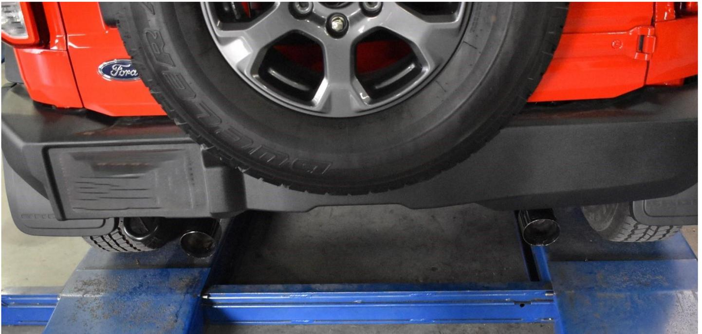
*Note: When you first start your vehicle after the installation of your new Ford Performance Parts Exhaust System, there may be some smoke and fumes coming from the system. This is a protective water-based coating used in the manufacturing of mandrel bent performance exhaust tubing. This is not a problem and will disappear within a very short period of time after the exhaust has reached operating temperatures.*
