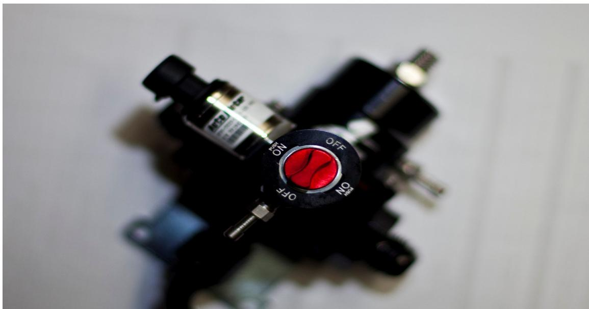
Taking a sample will require a length of 5/32" fuel proof rubber hose to reach whatever vessel being used to hold the sample. After installing the sample hose, with the vehicle master cutoff switch on, turn on the
