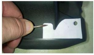
Step 5. Cut 1" hole with center in the marked location. A 1" drill or 1" hole saw may be used.
