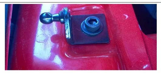
Step 7. Reinstall the battery cover and reinstall the push pins that secure the battery cover in place.
