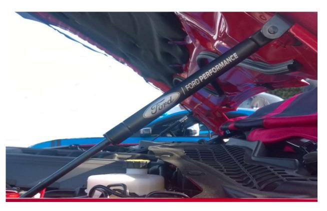
Step 9. Test function of hood struts Step 10. Remove hood prop from radiator support cover.
