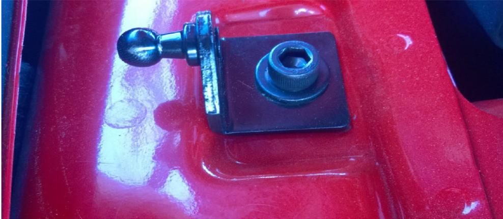
**Step 7. Reinstall the battery cover and reinstall the push pins that secure the battery cover in place.**
