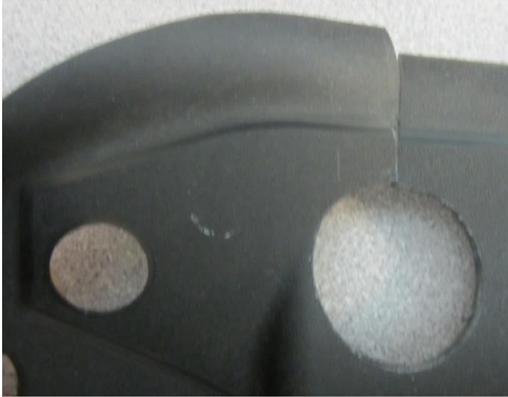
**Step 6. Place assembled lower bracket retainer into the fender hole by sliding the retainer inside the hole (drivers side has the lock washer, two retaining pins and star washer).**
