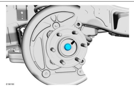
Position the wheel speed sensor wire and clip the 2 wheel speed sensor wire retainers.
