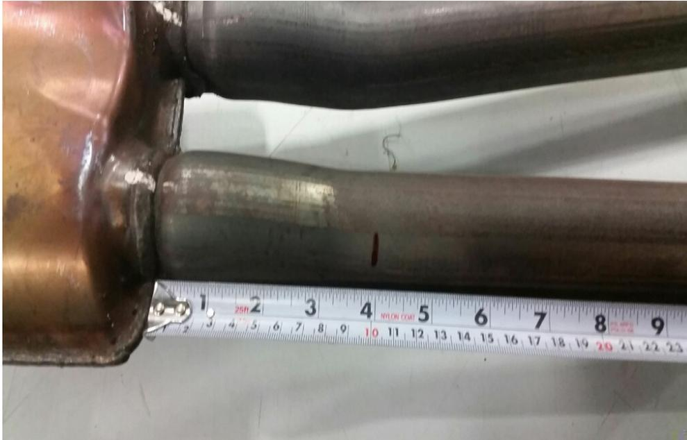
**STEP 6:** Slide the X-pipe into RH catalytic converter and LH muffler inlet pipe clamps. Making sure to center the clamps between the two pipes. Snug both clamps to hold X-pipe in place.
