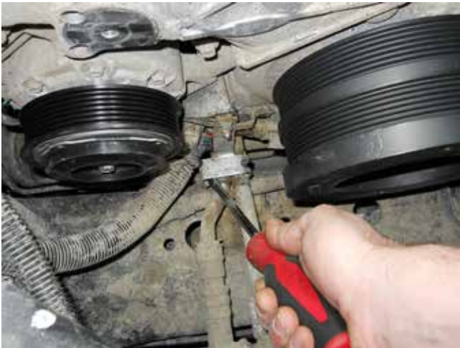
3. Remove the bolt from the bracket.
