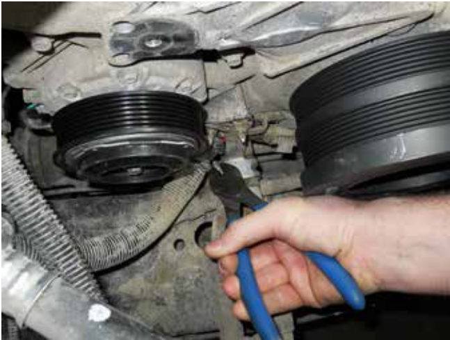
2. Bend the flat part of the bracket apart.
