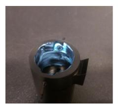
**STEP 27:** Install the lower O-Ring removed in Step 7, then slide the new reverse lockout collar onto the shifter shaft.
