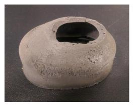
**STEP 31:** Install the OEM foam insulator over the shifter assembly and verify there is no interference with the reverse lockout collar.
