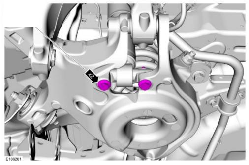
4.4 Remove the 2 rear shock absorber upper bolts and remove the rear shock absorber.
