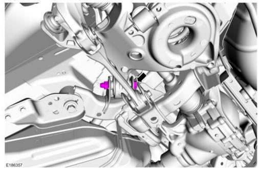
18.3 Tighten the toe link to frame bolt, ensuring the cam is in the correct position. Torque: 129 lb.ft (175 Nm)
