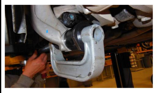
9.2 With the old bushing removed, set up your ball joint press with new bearing to press in knuckle.
