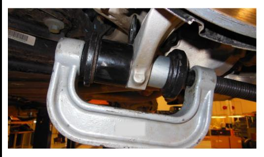
9.3 Press in new bearing and ensure bearing is centered in knuckle.
