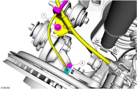
14.3 Install the lower bolt for the integral link to the lower control arm (labeled 2 below). Apply Loc-Tite to bolt and tighten to torque. The upper bolt should have been left attached.
