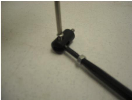
**STEP 8:** Apply a liberal amount of Blue thread locking compound on upper stanchion thread and proceed with installation. Install upper stanchion without support rod into the bumper bracket. This is done from below the vehicle, behind the lower grill.
