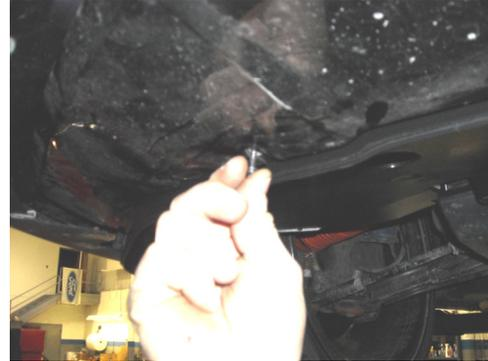
**STEP 3:** Remove the (4) bolts on the forward edge of belly pan to fascia. Remove belly pan from vehicle.
