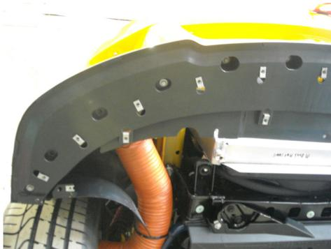
**STEP 5:** Remove the (2) Phillips screws that retain the support rod to the stanchions and separate.
