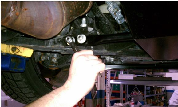
**STEP 34:** Torque (4) nuts to 35 ft.-lb. Note: Transmission cooling scoop is pictured (Blue) for clarification.
