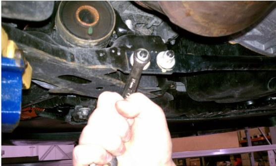
**STEP 31:** Remove the rear support brace from the sub frame studs.
