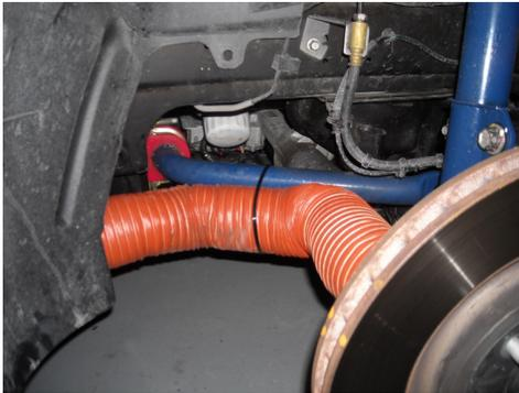
**STEP 20:** Slide the brake hose over the new backing plates and secure with provided hose clamp.
