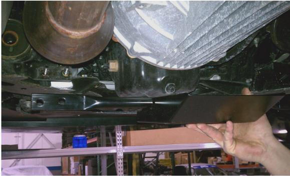
**STEP 33:** Install the (4) nuts onto the sub frame studs with Blue thread locking compound and tighten.
