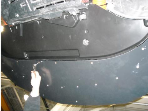
**STEP 28:** Install the splitter support rods to the splitter and torque bolts to 28 in.-lb.
