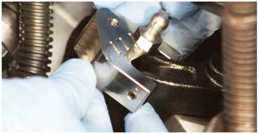
STEP 8: Use the supplied cap head bolt to pass through the original pin hole and tighten into the new billet body from beneath using an allen key. Tighten both pinch bolts on either side with an allen key.
