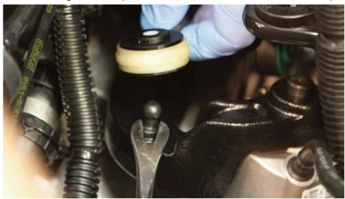
STEP 6: Using the supplied puller tool, hook the end over the pin and wind the nut until it locks against the sleeve as shown - continune to tighten until the pin is pulled from the standard arm.
