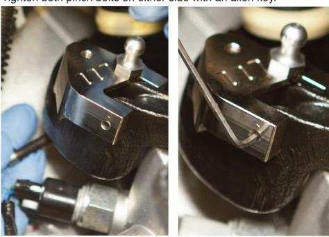
STEP 9: Push shifter cable end onto the new pin and check shifter engagement from the cabin. Re-fit airbox in reverse procedure to removal.
