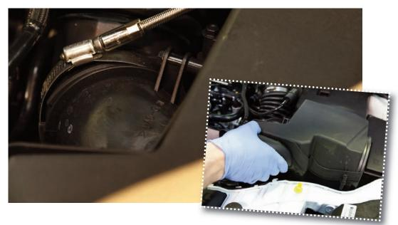
STEP 3A: Separate the upper symposer pipe - it pulls off. - Go to STEP 5 (FOCUS)
