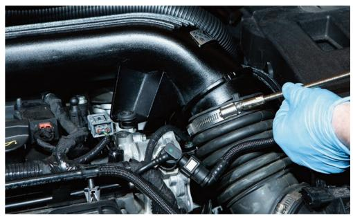
STEP 9: Re-fit the airbox lid, make sure the new hose connections are tight and then re-fit the engine cover
