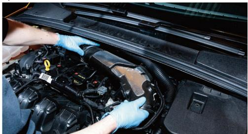
STEP 5: Remove the rubber gromit from the standard crossover and re-fit to the new mountune low-loss crossover, as shown
