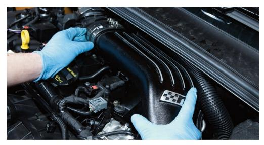
STEP 7: Remove the airbox lid by undoing the 4 retaining screws, then replace the standard filter element with the new K&N 57S filter - a detatchable plug is supplied with the filter should you require this for homolgation, optimum performance is achieved wih the plug removed
