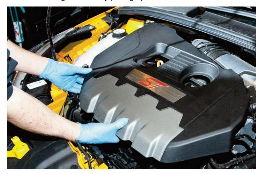
STEP 2: Undo the bolt securing the standard crossover duct in-situ with the cam cover
