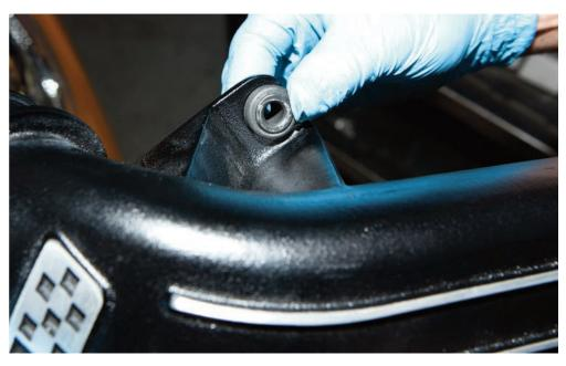
**STEP 6:** Your new crossover is supplied with a silicone hose and clips, make sure the clips are arranged in the orientation shown to avoid fouling
