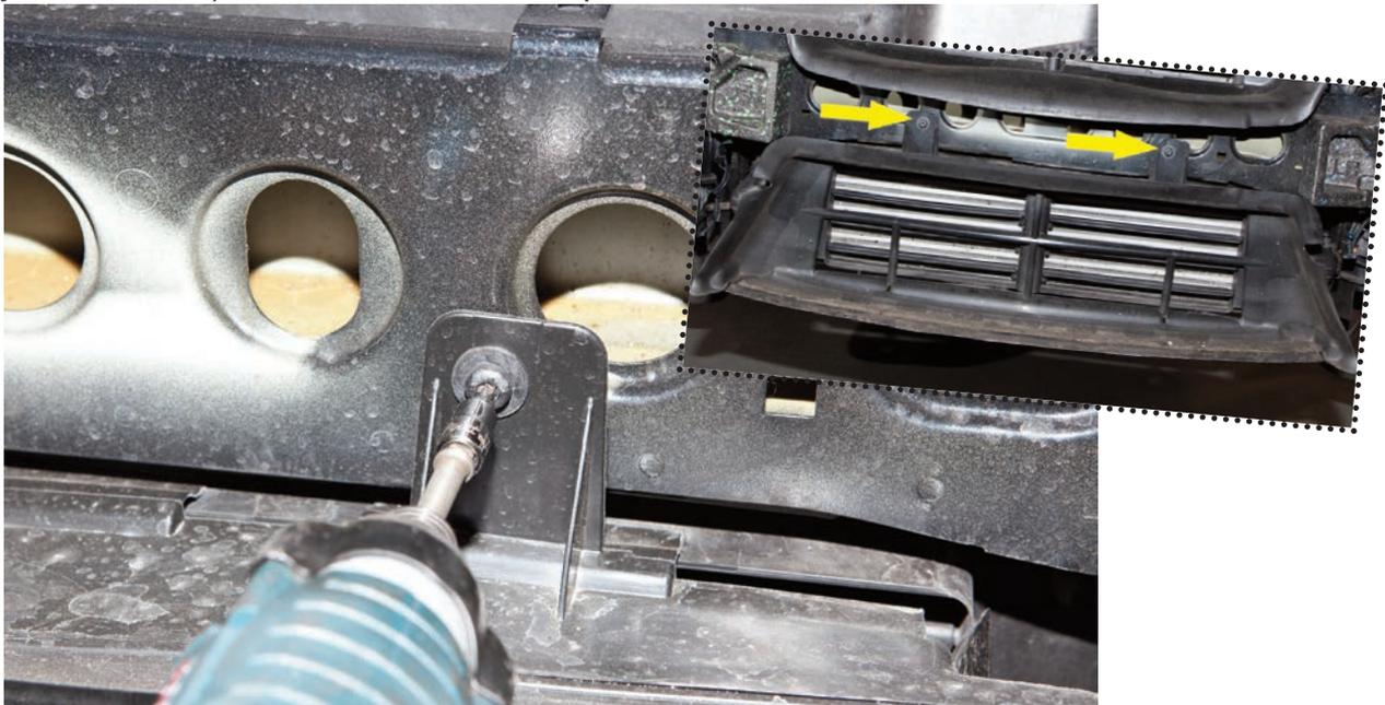
**STEP 11:** You'll now have access to the 'active grill shutter' - this needs to be removed later but at this point push the blades to ensure it's in the fully closed position
