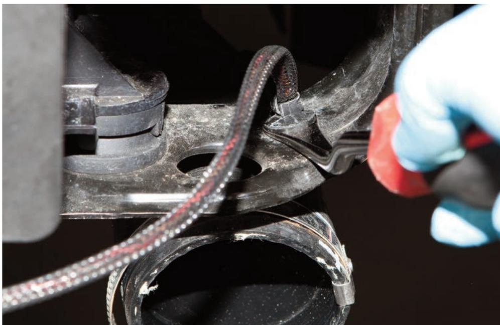
**STEP 23:** Manouver the AGS free of the two clips on either side and then remove the complete assembly
