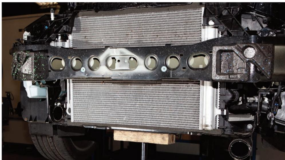
**STEP 28:** Remove the radiator cradle bolts on both sides
