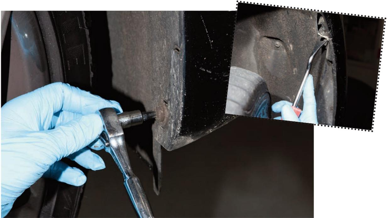
**STEP 6:** A) Undo and remove the lower deflector B) Remove the rear section of the undertray C) Undo and remove the corner deflector as shown
