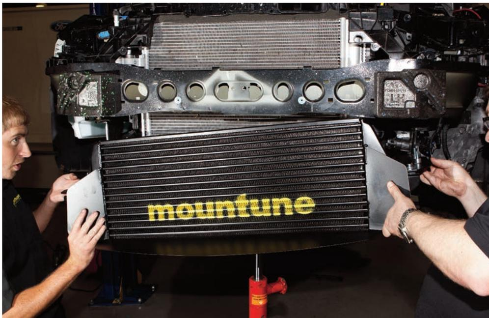
**STEP 30:** The side brackets fit underneath the radiator cradle as shown in STEP 30 and 31
