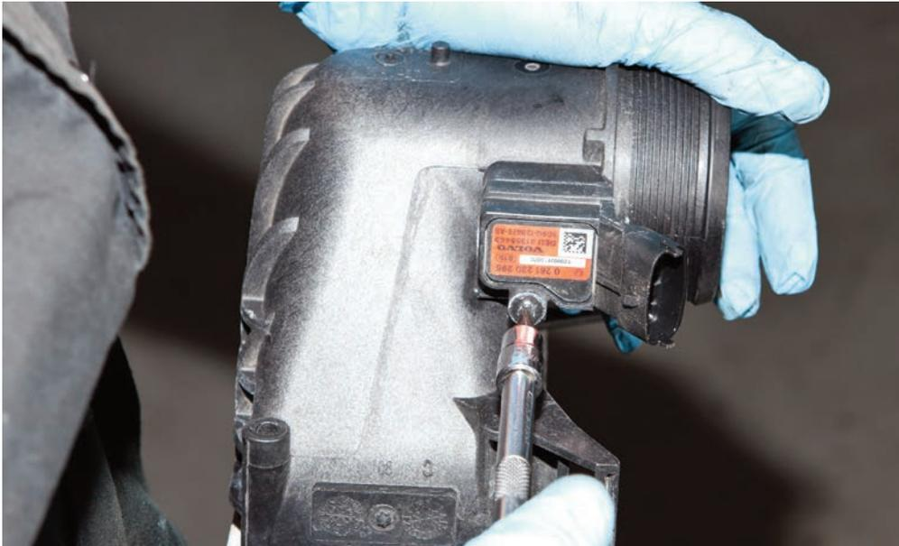
**STEP 20:** Re-fit this to the new intercooler as shown. Note: US intercoolers will require an additional bracket (supplied) to hold the MAP sensor in the correct orientation
