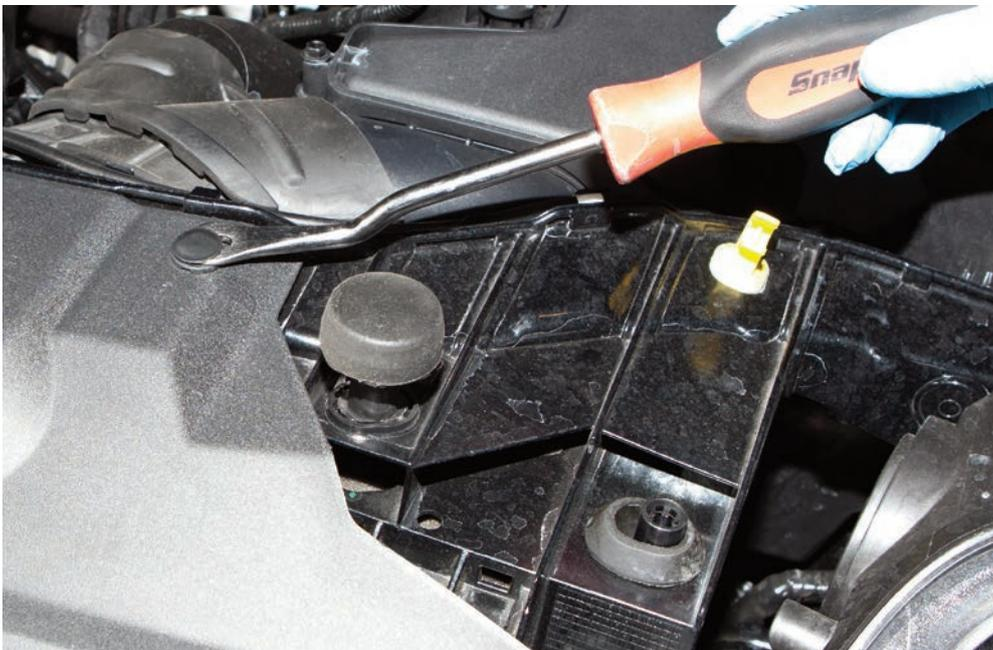
**STEP 2:** Disconnect the bonnet release cable and then withdraw the top cover
