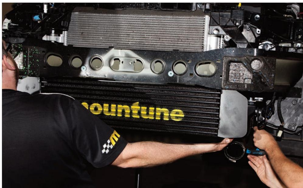
... then fully tighten the cap head bolts. Note: the shorter bolt is used on the LHS
