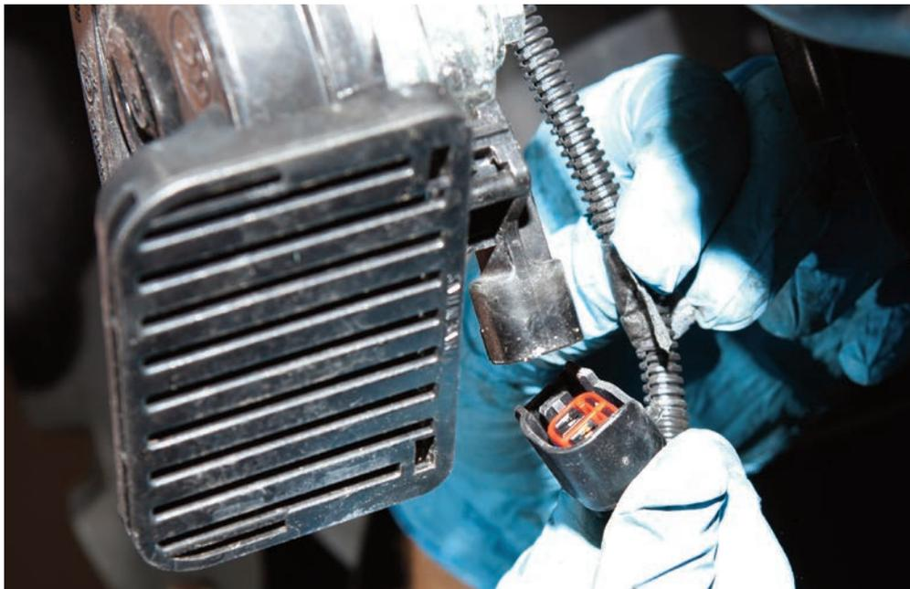
**STEP 16:** Use a trim tool, or similar, to free horn loom mounting clip
