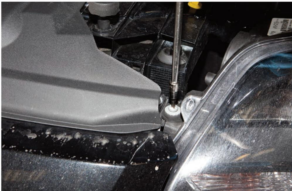
**STEP 4:** Pull the headlight's upwards to remove it from its mount. You'll need to disconnect the plug as shown
