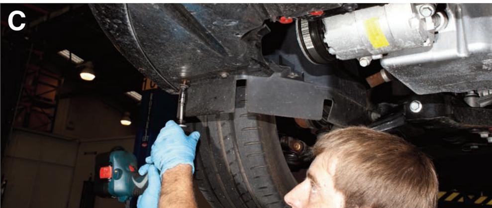
**STEP 7:** Undo the two bumper bolts (by headlights). Then unclip the front bumper from the wing on both sides
