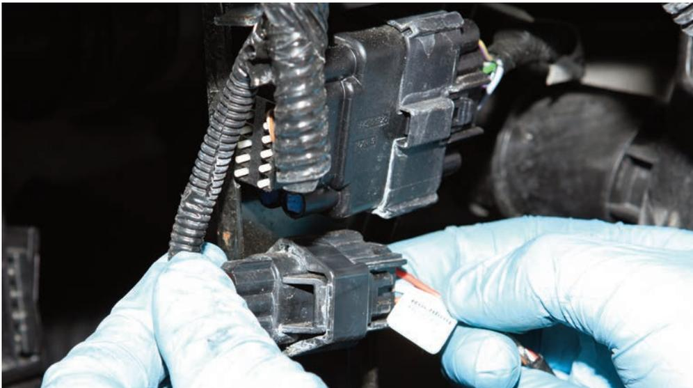
**STEP 22:** Using a trim tool, or similar, free the AGS loom
