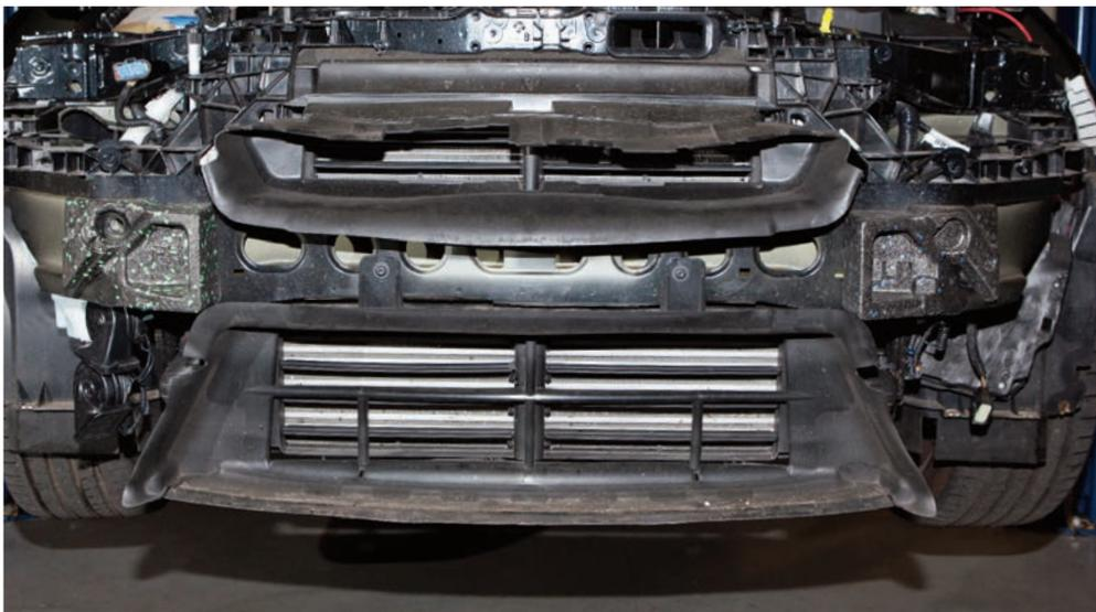
**STEP 9:** Pull the top air duct free from its mounting locators
