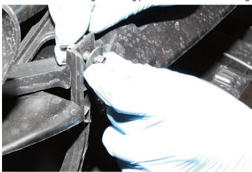
STEP 12: Undo the three bolts supporting the lower cooling pack cradle
