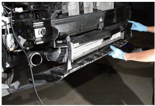
STEP 14: Undo the intercooling mounting bolts on both sides
