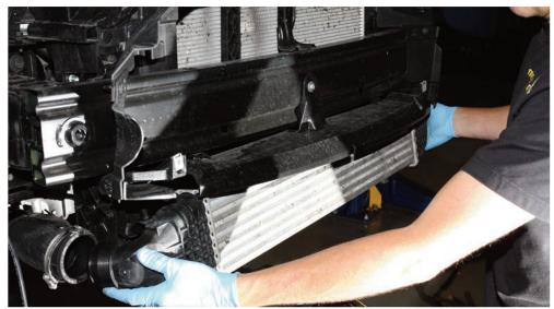
STEP 16: Install the mountune intercooler by reverse procedure - ensure the rubber locating mounts are transferred across
