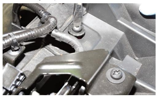
**STEP 9:** The bumper can now be removed by pulling forwards - as shown
