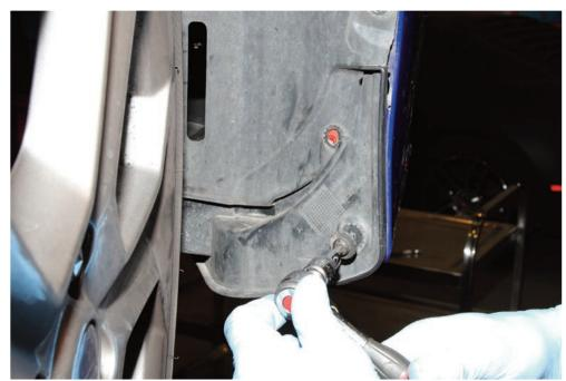
STEP 7: Underneath the car, undo the fasteners holding the cooling pack cradle to the bumper
