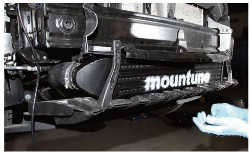
**STEP 20:** The front of the car should now look like this; re-fit the bumper and headlights by the reverse procedure to instalation.
