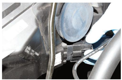
STEP 4: Undo the foglight connectors on both sides via the access created by removing the headlights
