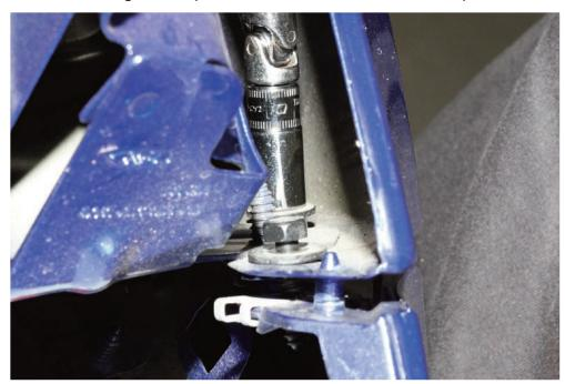
STEP 6: Undo the fasteners holding the wheel arch liner to the bumper on both sides
