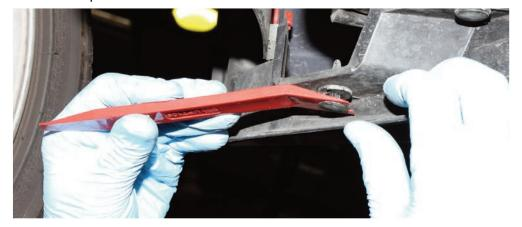
STEP 8: Undo the remaing slam panel cover bolts next to the bonnet release catch
