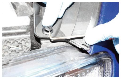
STEP 3: Withdraw both headlights by pulling upwards - once lifted partially out of place you'll be able to undo the electrical connector on the rear
