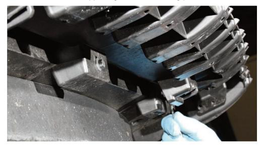
STEP 13: Carefully withdraw the lower cooling pack cradle as shown
