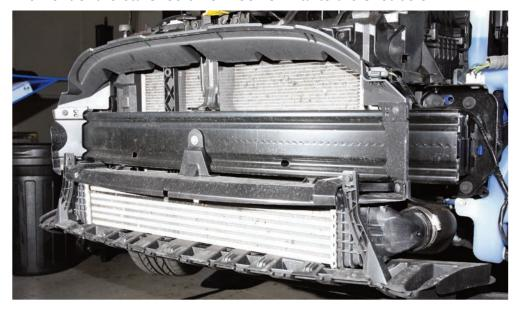
STEP 10: Undo the jubilee clip holding the boost pipe and withdraw (repeat on opposite side)
