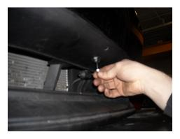
**STEP 5:** Install the splitter support rods onto rod ends; torque bolts through splitter to 28 in.-lb.
