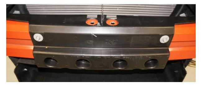
The Hole cut in the Radiator Air Deflector will allow clearance for the upper spacers and the Nut on the bottom of the Bumper Beam.
