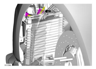
Disconnect the Electrical Connectors for the Turn Signals and Running Lamps on both sides
