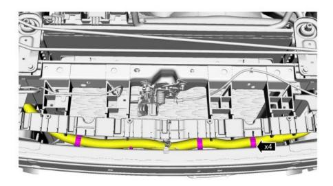
Separate the wiring harness guides.
