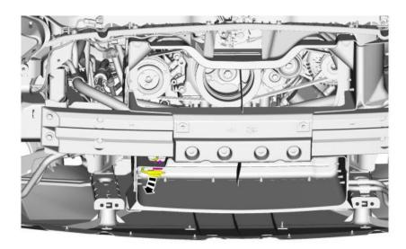
Position aside the ambient air temperature sensor bracket.
