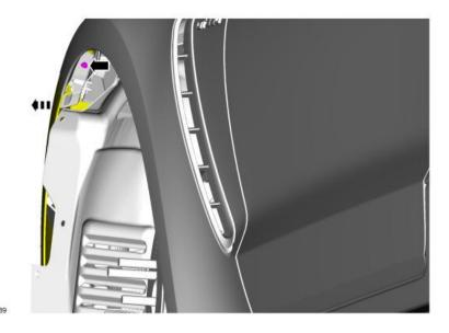
Remove the Screw and separate the Front Bumper from the retention clip on both sides
