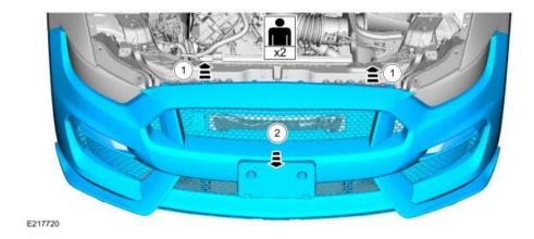
With the assistance of a Helper, lift the fascia up and off the Location Pins, then forward. The Front Fascia and Under Tray will come off as a single unit.
