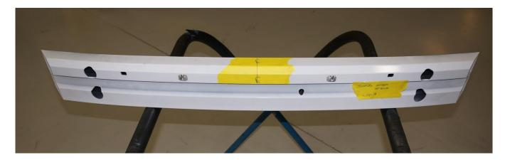
Find Center on the Bumper Beam and Mark a Line as shown above.
