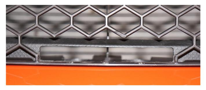
Find the Vertical Centerline of the Upper Grille. At the Bottom of the Grille, remove the Honeycomb as shown above. The section of Grille to be removed will be ¾ inch tall by 4 Inches wide. Also, behind the Grille, notice the trim piece that is modified as well. This piece also needs to be trimmed to 4 inches wide but only as tall as necessary to leave the top and bottom in place.
