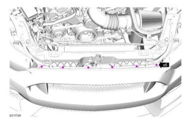
Remove the six (6) Screws along the top of the Front Fascia
