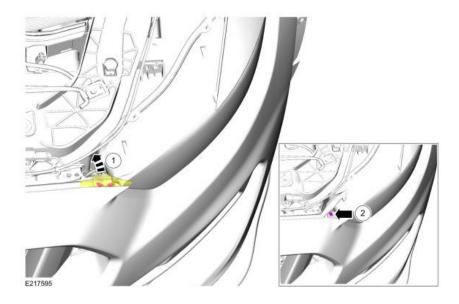
Remove the screws under the Hood Leading Edge Seal
