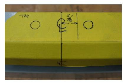
The Beam should look like the above Picture. Drill the two 7/16 Holes completely through the Bumper Beam. There are Three (3) layers to go through. It is highly recommended that you drill these Holes on a Drill Press. This will ensure all three layers are aligned and straight.
