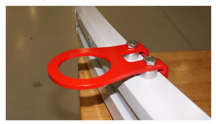
Install the Front Tow Ring using the provided Hardware. Insert the bolts through the Ring, install the Spacers next then, install the Ring Assembly on the Bumper Beam, through the holes cut in the Radiator Air Deflector. Install the Supplied Lock Nuts.
