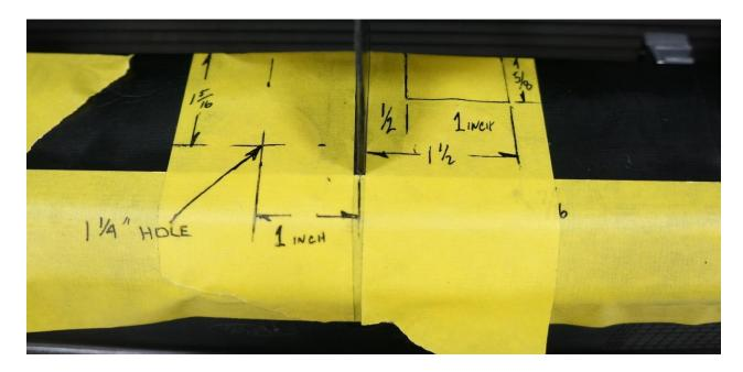
The Radiator Air Deflector needs to be modified next. In the Pictures above and below are the two different types of modifications necessary. For the Tow Ring Mounting Reliefs, use the measurements on the Left to locate the center point for the 1 ¼ inch hole on both sides of the Center Divider. Use the measurements on the Right to mark the Notch that needs to be cut out of the Deflector on both sides of the Center Divider. This will need to be done above and below the bumper beam.
