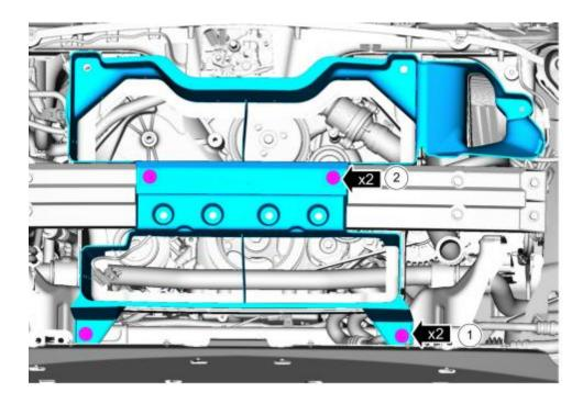
Remove the bolts and the radiator air deflector.
