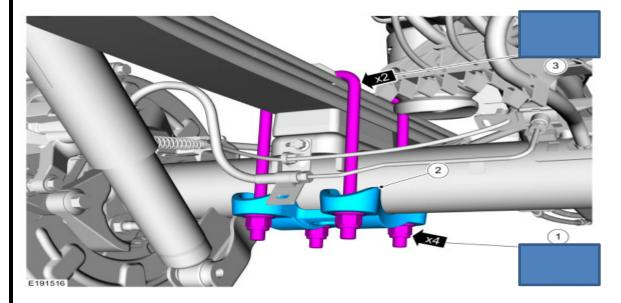
For the <u>LH</u> spring. Lower the fuel tank to gain access to the spring-to-frame bolt.
