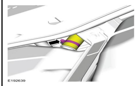
2.Insert the hose from the Fuel Tanker (NOT INCLUDED) and siphon the fuel through the fuel tank inlet spout.
