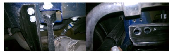
**NOTE:** Lubricate the muffler assembly isolators with soapy water to ease in removal.
