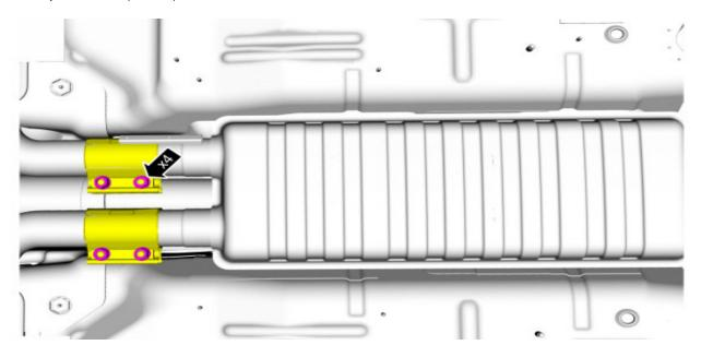
STEP 4: Remove the <u>LH</u> and <u>RH</u> rear exhaust hanger isolator bracket bolts. Unhook the rear exhaust hanger isolators and remove the muffler and tailpipe. *Torque*: 18 lb.ft (25 Nm)
