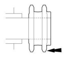
**STEP 13:** Position the LH (inner) timing chain on the crankshaft sprocket, aligning the copper (marked) link with the timing mark on the sprocket.
