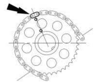
**STEP 20:** Position the RH timing chain tensioner arms on the dowel pin and install the RH timing chain tensioner.
