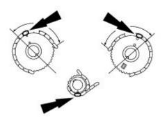
!!! CAUTION: Unless otherwise instructed, at no time when the timing chains are removed and the cylinder heads are installed is the crankshaft or the camshaft to be rotated. Severe piston and valve damage will occur if cam followers are installed. !!!
