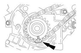
**STEP 14:** Install the LH timing chain onto the crankshaft sprocket, aligning the copper (marked) link with the timing marks on the sprocket.
