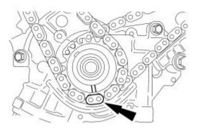
**STEP 19:** Install the RH timing chain onto the crankshaft sprocket, aligning the copper (marked) link with the timing marks on the sprocket.
