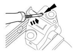
**STEP 5:** While holding the ratchet mechanism, push the ratchet arm back into the tensioner housing.
