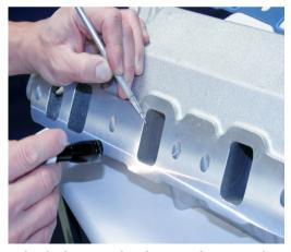
5. Test fit the carburetor/throttle body and actuate the linkage. Check to make sure the throttle blades do not contact the manifold.
