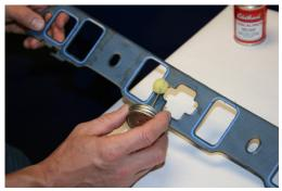
13. Install EGR gasket or block-off, depending on intake manifold style. If the manifold does not have an EGR passage (no EGR passage on our example) the block-off is used.
