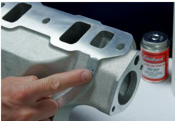
15. Apply a thick layer of silicone onto the end rails of the block, be sure to apply in corners.
