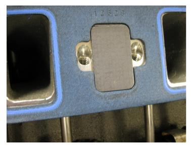
14. Rub an initial thin layer of silicone onto the end rails of the intake manifold <u>and</u> block.
