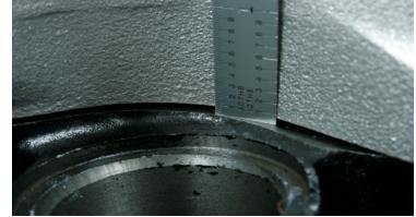
• If the gap is less than .040" the end rails of the manifold will need to be machined. This can be checked with a scale or feeler gauges.
