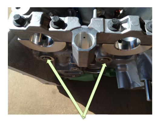
Factory 5.2L GT350 heads come with two 1.275mm oil restrictors installed in the front of each cylinder head.
