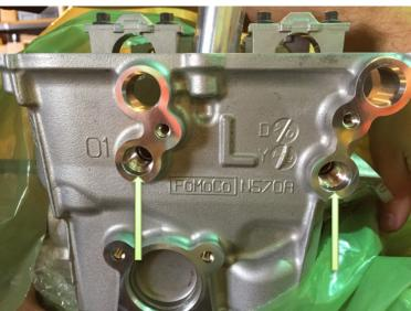
Remove pipe plugs from the rear of cylinder heads.
