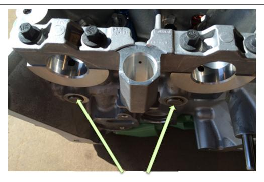
Tap the restrictors into the cylinder head with a brass hammer and they will bottom out with slight protrusion as seen above.
