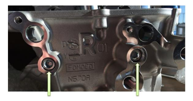
Install new pipe plugs provided and torque to 10lbft + 180deg of rotation.
