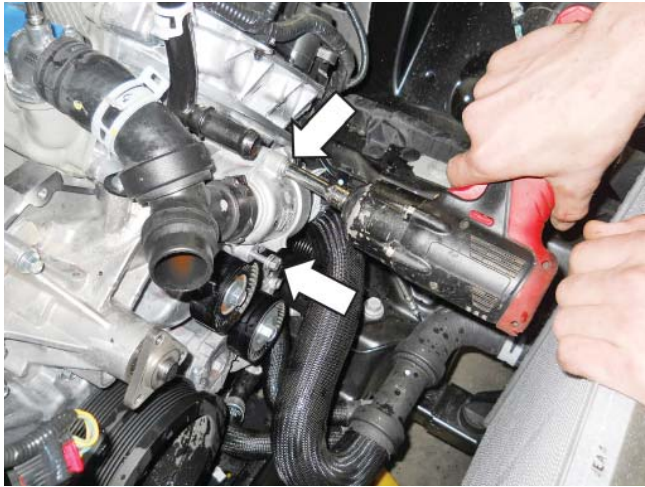
53. Remove the thermostat housing assembly and set it aside.
