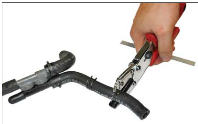
18. Insert the brake booster check valve on the end of hose 2 and secure it with the clamp.
