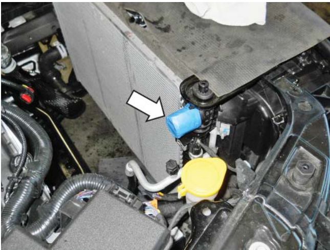
57. Tape off the radiator hose port and inlet port.
