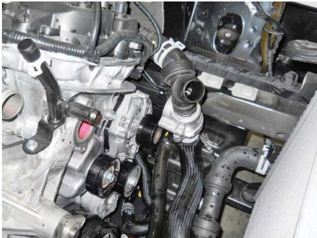
54. Remove the four (4) water pump mounting bolts (10 mm socket) and remove the water pump. Set both aside for re-use.
