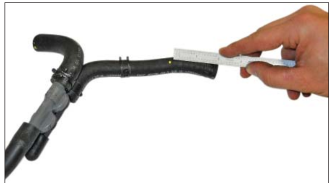
17. On hose 2, mark and cut 2" from the end of the hose.
