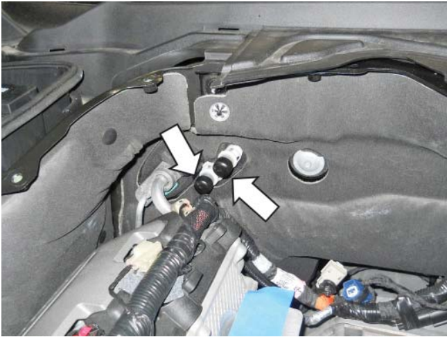
57. Tape off the radiator hose port and inlet port.
