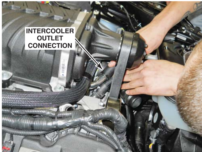
Outlet hose connection at top port of intercooler
