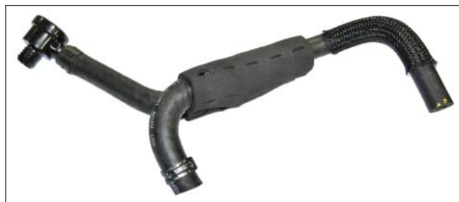
20. Re-wrap the foam sleeve on the modified brake booster hose and aspirator assembly as shown.
