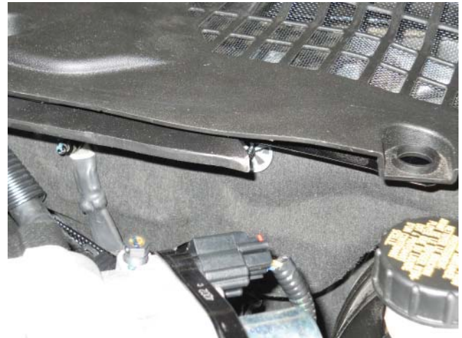
Exposed point on modified K-brace, shown installed
