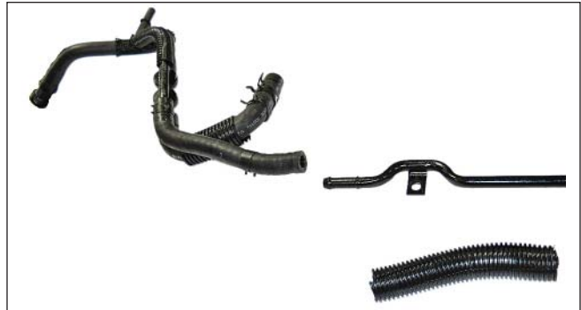
10. Remove the convolute from the curved nylon tube (hose 5).
