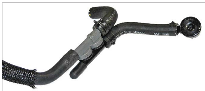
19. On hose 3, trim 3/4" past the radius on the bend shown. This hose will connect to the clean air tube.
