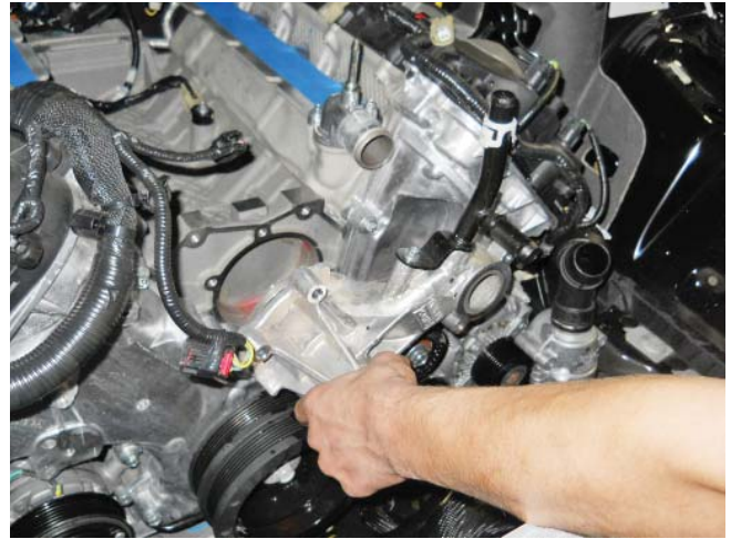
55. Place a clean towel in the water pump inlet cavity.
