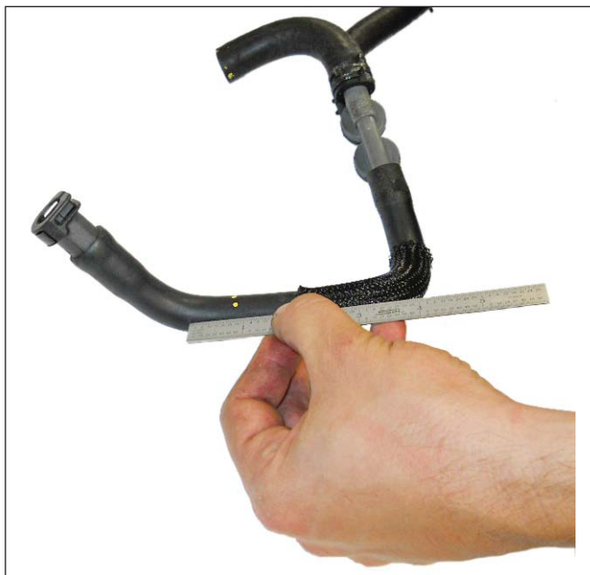
19. On hose 3, trim 3/4" past the radius on the bend shown. This hose will connect to the clean air tube.
