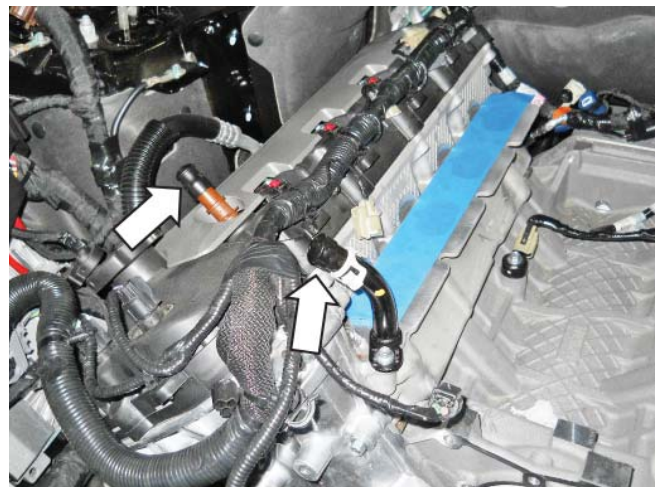
56. Cap or tape off the PCV port, heater feed tube and the heater core ports on the firewall.
