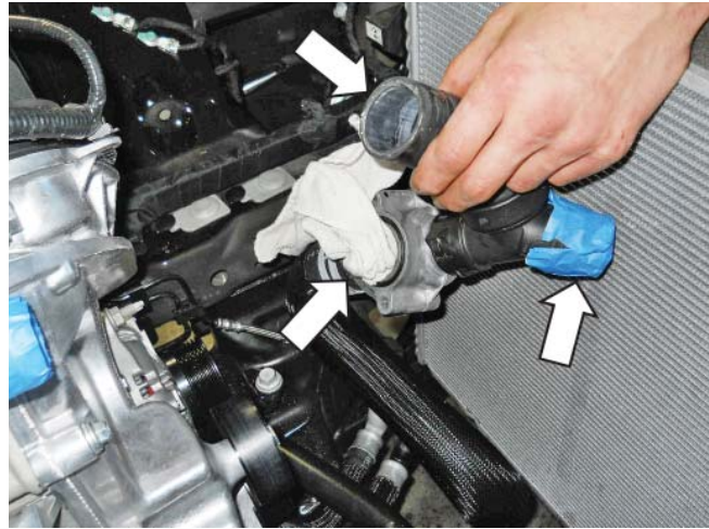
58. Tape off and block the thermostat housing ports. Use care to prevent coolant from leaking from the housing and hose.
