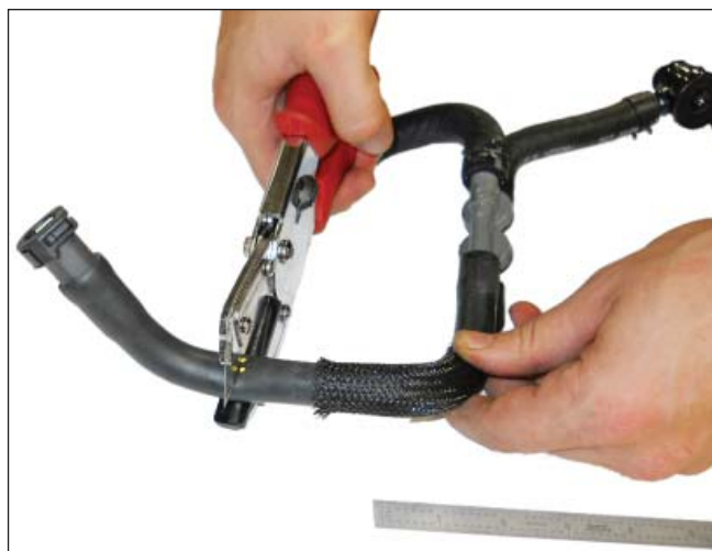
20. Re-wrap the foam sleeve on the modified brake booster hose and aspirator assembly as shown.
