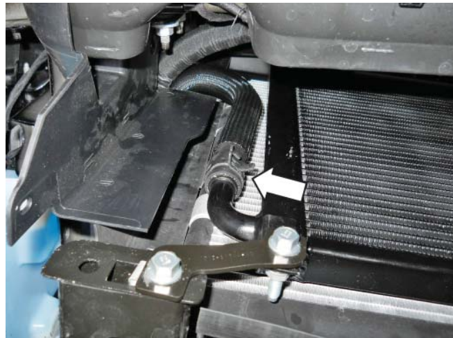
Pump hose to LTR connection
